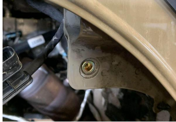
Install the riv nut at existing thru hole, on left and right side upper rear location (Driver side shown)
