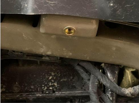
Install the riv nut at existing thru hole, on left and right side forward upper support bracket (Driver side shown)
